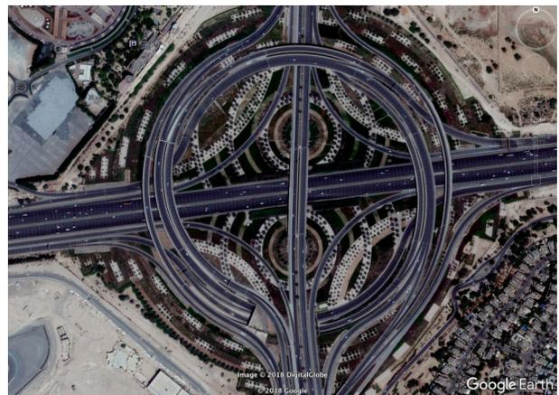
Figure 3 – Truck Friendly Large Roundabout, Dubai
