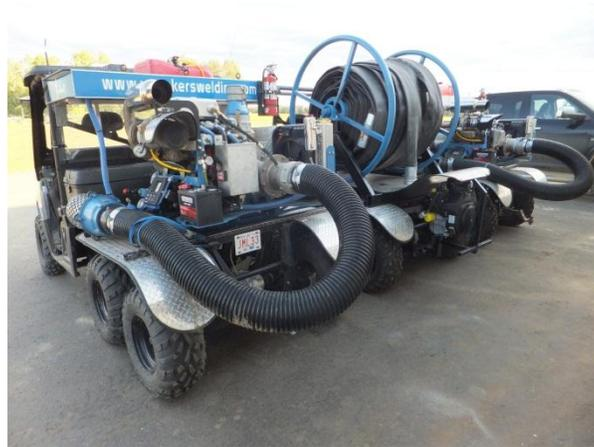
The Trident's dry weight is 500 lbs. It's most powerful model can output 10,000 Imperial gpm, but the pump in the video was designed to flow 3,000 Imperial gpm.
